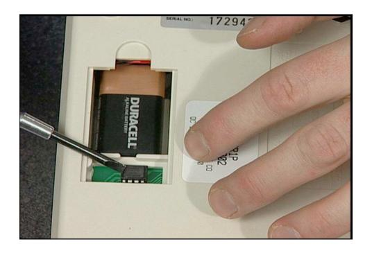
Note the direction of the old chip. You will see the notch on the top surface of the chip.
